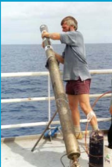
**Scientist loading a sonobuoy into a compressed air launcher**
