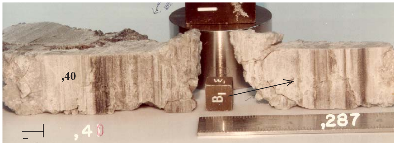
Figure 27: 61016,40 after sawing off the top (287). Small cube is 1 cm. NASA S74-33206. Streaks are from saw blade.
