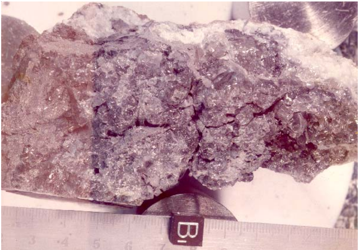
Figure 30: Plagioclase glass boundary on bottom surface of 61016,98. Cube is 1 cm. NASA S75-33581.
