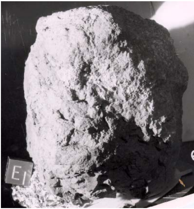
Figure 2: Photo of E1 side of 61016 with lighting similar to lunar lighting, thus providing knowledge of lunar orientation. Cube is 1 inch, showing approximate lunar orientation. NASA#S72-41841
