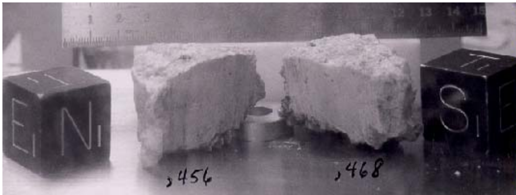
Figure 32: Saw cut through 61016,456, producing ,468. Cube is 1 inch (cm scale in background). Photo from data pack.
