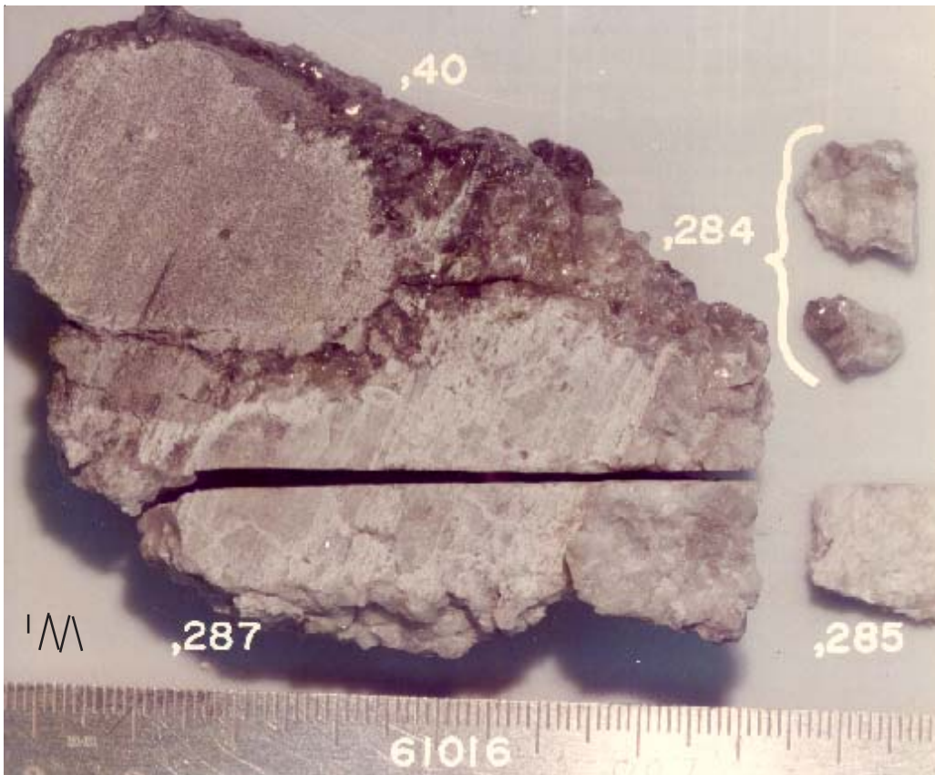
Figure 26: Photo of top portion of slab from 61016 (with T1 surface facing the ruler). NASA S74-33208. Scale in cm. Compare with figure 5 (top piece).
